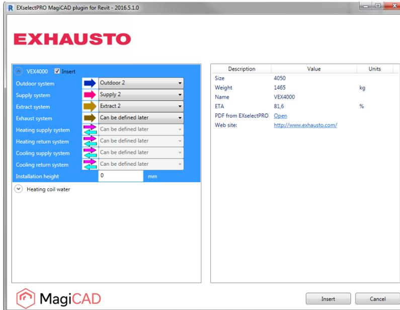
Please note that the Import operation takes longer the first time when the air handling unit is converted to RFA format. When the same air handling unit is imported again to the Revit project, the Import feature works much faster.
